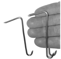
Don't do this The above strap technique is undesirable for two basic reasons: it looks bad and the straps are easily bent open by sliding ice and snow.
